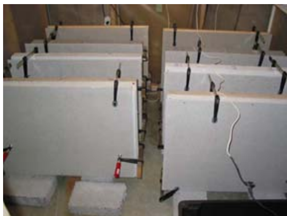
FIG. 3: The tested exterior wall assemblies in the climate chamber (on the left). The principle of the test specimen (on the right).
