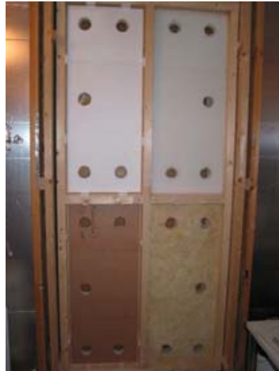
FIG. 4: The test building (on the left) and the wall module which is divided into four different exterior wall assemblies (on the right).
