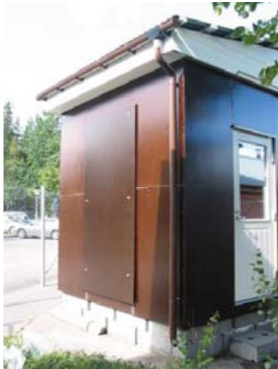
FIG. 4: The test building (on the left) and the wall module which is divided into four different exterior wall assemblies (on the right).
