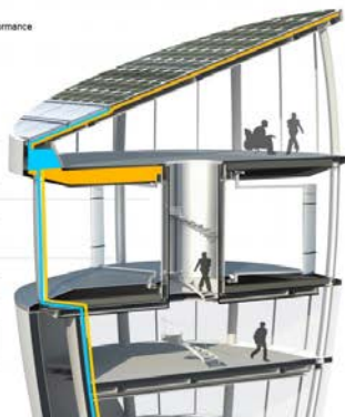
Figure 6. Turbine-House design and renewable energy systems integration.
