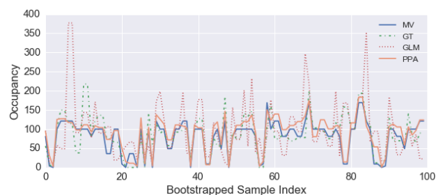
Figure 6: Ground Truth (GT) and predictions using the above described techniques. Poisson Regression (GLM) performs considerably worse than the GMM-HMM models.
