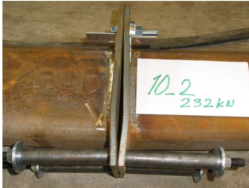
Figure 2.11. Specimen 10_2 after the test.
