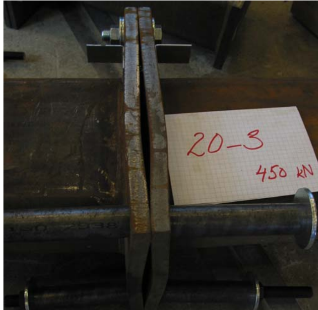
Figure 2.32. Specimen 20_3 after the test.
