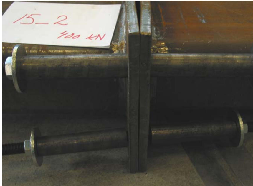
Figure 2.20. Specimen 15_2 after the test.
