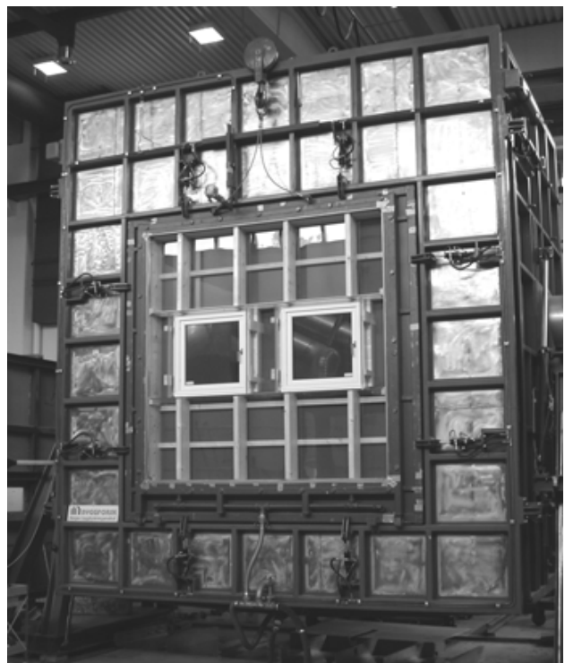
Figure 3b Test area undergoing driving-rain tests in a RAWI-box (turnable equipment for full-scale RAin and WInd tightness testing).
