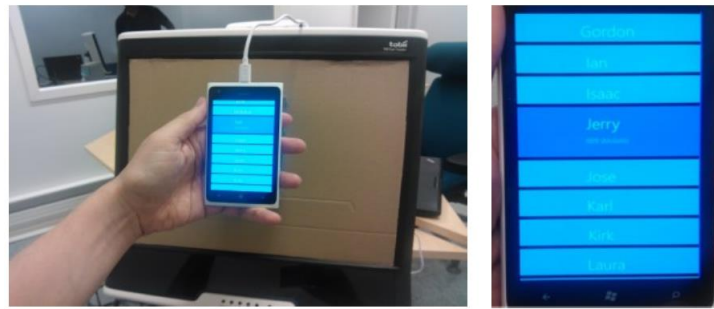
FIGURE 3. The mobile phone used in Kangas et al. (2014b) was held in front of a gaze tracker (left). The experimental interface consisted of a list of contact names (right). © 2014 Association for Computing Machinery, Inc. Reprinted by permission.
