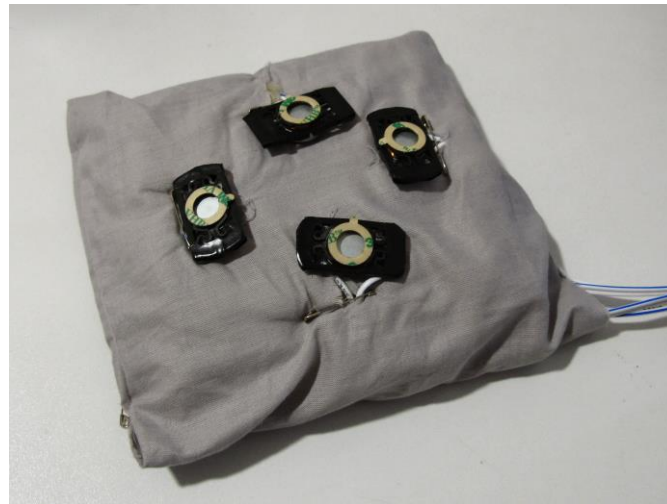
FIGURE 13. Pillow with four actuators used in the study by Köpsel et al. (2016).
