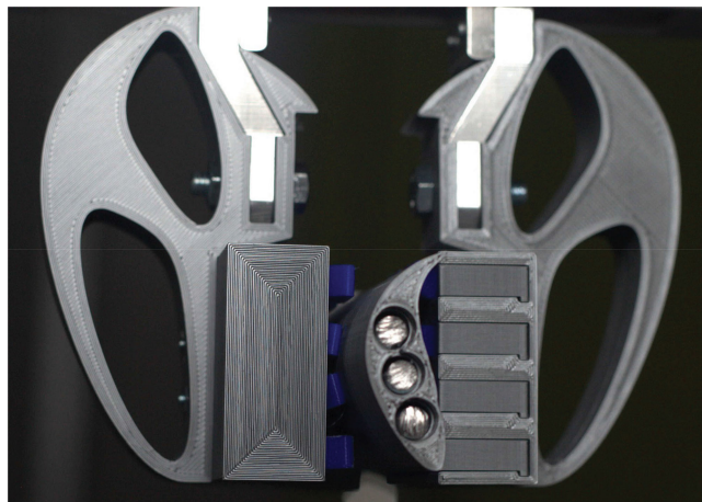
Fig. 1. Soft gripper design (grey) with compliant structures (blue) successfully holding a mock turbojet turbine blade (grey curved object with three weight inserts). The compliant structures deform to the shape of the object, which would not be possible with a rigid parallel gripper.
