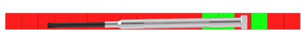
(f) The small screwdriver (stainless steel, 0.02kg) only has few successful grasps, likely due to its size being small enough to slip in between cells.
