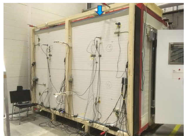
Fig. 1. Wall tests at HAMK Tech. Blue arrow points the location, where additional water was injected during the tests. Radio transceivers were installed close to the exterior corners of each element.
