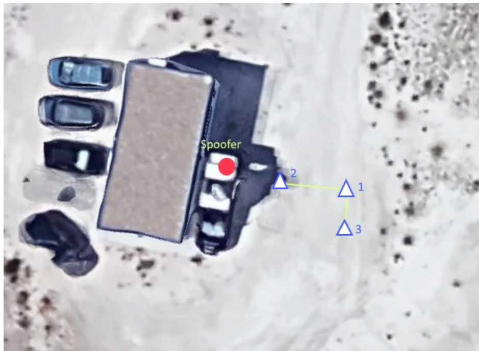
Figure 8. OF-SPO-Z2-S-Test 1 and 5: Open field static configuration of the transmitting and receiving antennas.
