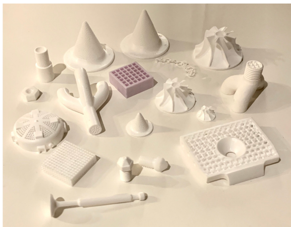
Fig. 7. Ceramic parts manufactured by using CeraFab 7500 at Tampere University (Credit goes to Teemu Vastamäki and Jorma Vihinen for the fabrication of these parts).
