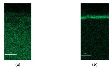
**Figure 6.** Elemental mapping of Ag in Ag2 (**a**) prior to and (**b**) and after heat treatment at the surface of samples.
