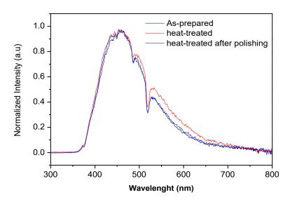
$\textbf{Figure 8.} \ \ \text{Normalized visible photoluminescence (PL) spectra of } \ \ \text{Ag}_2 \ \ \text{glasses taken as an example}.$
