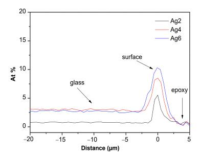
Figure 7. Ag concentration profile measured from the surface of the heat-treated glasses.
