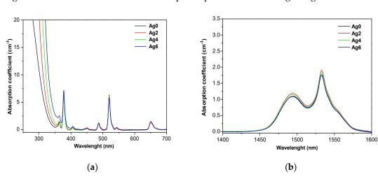
Figure 2. Absorption coefficient of the investigated glasses (a) in the UV-Vis and (b) IR range.
