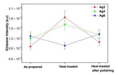
Figure 9. Variation of 1.53 μm band peak emission intensity.
