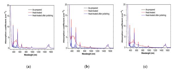
Figure 5. Absorption spectra of the heat-treated glasses: (a) Ag2, (b) Ag4, and (c) Ag6.
