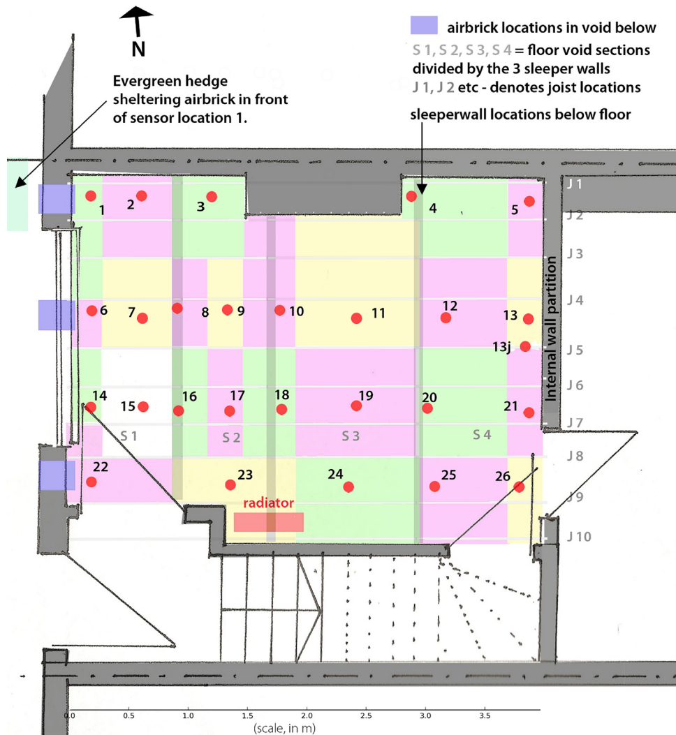
Fig. 1. Floor plan with heat flux sensor locations (red circles and numbered); airbrick locations (blue), and sleeper walls (grey). Approximate joist locations are marked with a faint grey line and annotated with J1, J2 etc. Location 13j is the only location measured on a joist. Portable radiant oil-filled electrical plug-in heaters are marked on the plan. Note that the colours have no meaning other than each colour distinguishes one representative area around a HF sensor from another. Representative areas were derived from infrared images. (For interpretation of the references to colour in this figure legend, the reader is referred to the web version of this article.)
