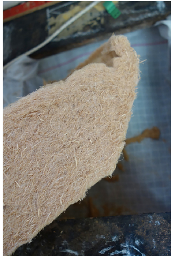
Fig. 5. Close-up of the chamfered woodfibre insulation to enable airbrick airflow.
