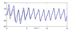
Fig. 9. Output (blue) of the beam model with the observer-based controller and the reference signal (gray).
