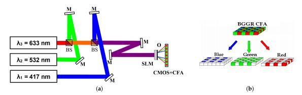
**Figure 1.** (a) Optical setup.  $\lambda_1 = 417 \text{ nm}$ ,  $\lambda_2 = 532 \text{ nm}$ ,  $\lambda_3 = 633 \text{ nm}$  are wavelengths of the blue, green, and red light sources, M are mirrors, BS are beam-splitters, SLM stands for Spatial Light Modulator, O is the object, CMOS+CFA is a registration camera with CFA; (b) Color filter array. BGGR CFA is a blue-green-green-red disposed CFA; Blue, Green and Red are separate color channels.
