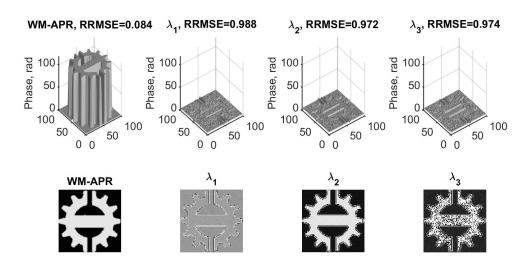
**Figure 6.** Logo TUT phase reconstructions: RRMSE = 0.084 (SNR = 6.3 dB,  $N_{photon} = 1.42$ ), (**top row**)—3D absolute phase surfaces, (**bottom row**)—the corresponding 2D absolute phases images. From left to right: WM-APR algorithm, and phase reconstructions obtained separately for  $\lambda_1$ ,  $\lambda_2$ ,  $\lambda_3$  wavelengths, respectively, followed by the 2D phase unwrapping.
