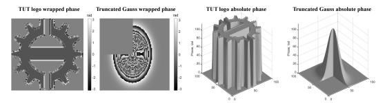
**Figure 2.** Wrapped and absolute phases of the investigated test-objects: truncated Gaussian and TUT logo, the reference wavelength  $\lambda' = \lambda_3$ .
