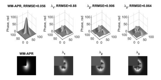
**Figure 5.** Truncated Gaussian absolute phase reconstructions: RRMSE = 0.056 (SNR = 6.3 dB,  $N_{photon} = 1.42$ ), top row - 3D absolute phase surfaces, bottom row - the corresponding 2D absolute phase images. From left to right: WM-APR algorithm, and phase reconstructions obtained separately for  $\lambda_1$ ,  $\lambda_2$ ,  $\lambda_3$  wavelengths, respectively, followed by the 2D phase unwrapping.
