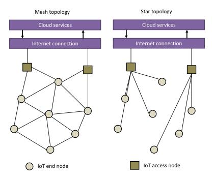
Figure 5. Comparison of a simplified IoT mesh and star network topology.
