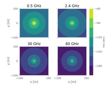
Figure 2. Ideal radio signal propagation at 0.5, 2.4, 30 and 60 GHz.
