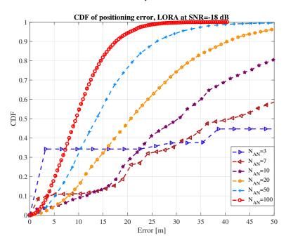
Figure 7. Example of LoRa performance at various numbers of access nodes.
