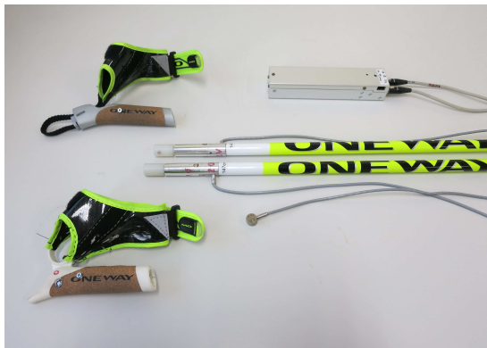
(a) A separate load cell can be seen below the poles. The data logger is above right. Above left is the standard grip and below left is the hinged grip. Both were used in the field tests.
