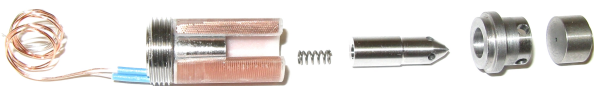
Figure 7. Each prototype valve consists of five turned parts, a coil and a spring.
