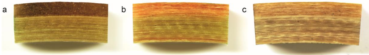
Figure 7: FRP-441 sample appearance (a) prior conditioning and after (b) 6 and (c) 12 months in 5% H_2SO_4 solution.
