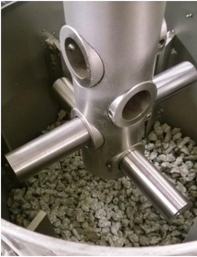
Figure 2: Dry-pot test configuration for the erosion wear tests. Before the test samples are submerged in to the abrasive bed.
