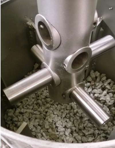
Figure 2: Dry-pot test configuration for the erosion wear tests. Before the start of the test samples are submerged in to the abrasive bed. The shaft rotates anticlockwise during the test.
