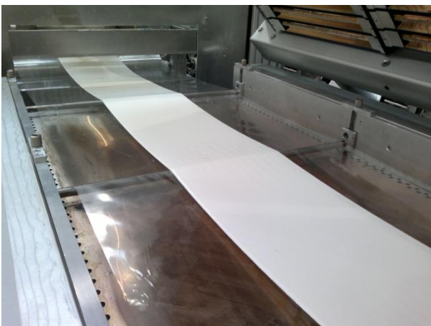
Fig.5 Smooth layer of pigment-CNF dispersion was spread on top of the support material.
