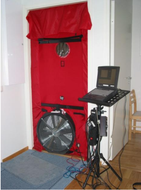
Figure 1. Blower-door system installed on door frames.
