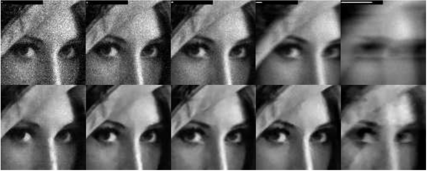
Fig. 5. Experiments on camera raw data: raw data images #1,2,3,5,8 with the estimated PSF (top row) and restored images (bottom row). Acquisition parameters and restoration performance are given in Table I. Images have been rescaled for visualization purposes.
