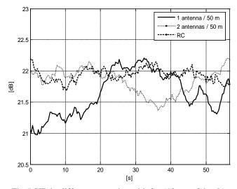
Fig.5 SIR in different scenarios with 8 s (10 m at 3 km/h) averaging window (sample rate 0.33 s).
