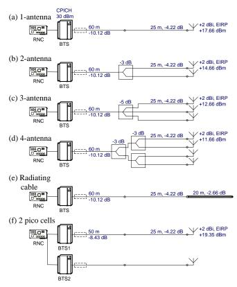
Fig. 2. Antenna lines for the different configurations.
