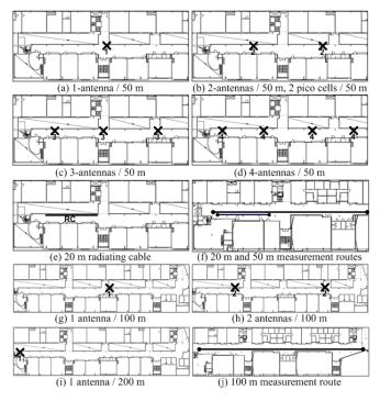
Fig. 1. Measurement routes and antenna placements for wide corridor measurements.
