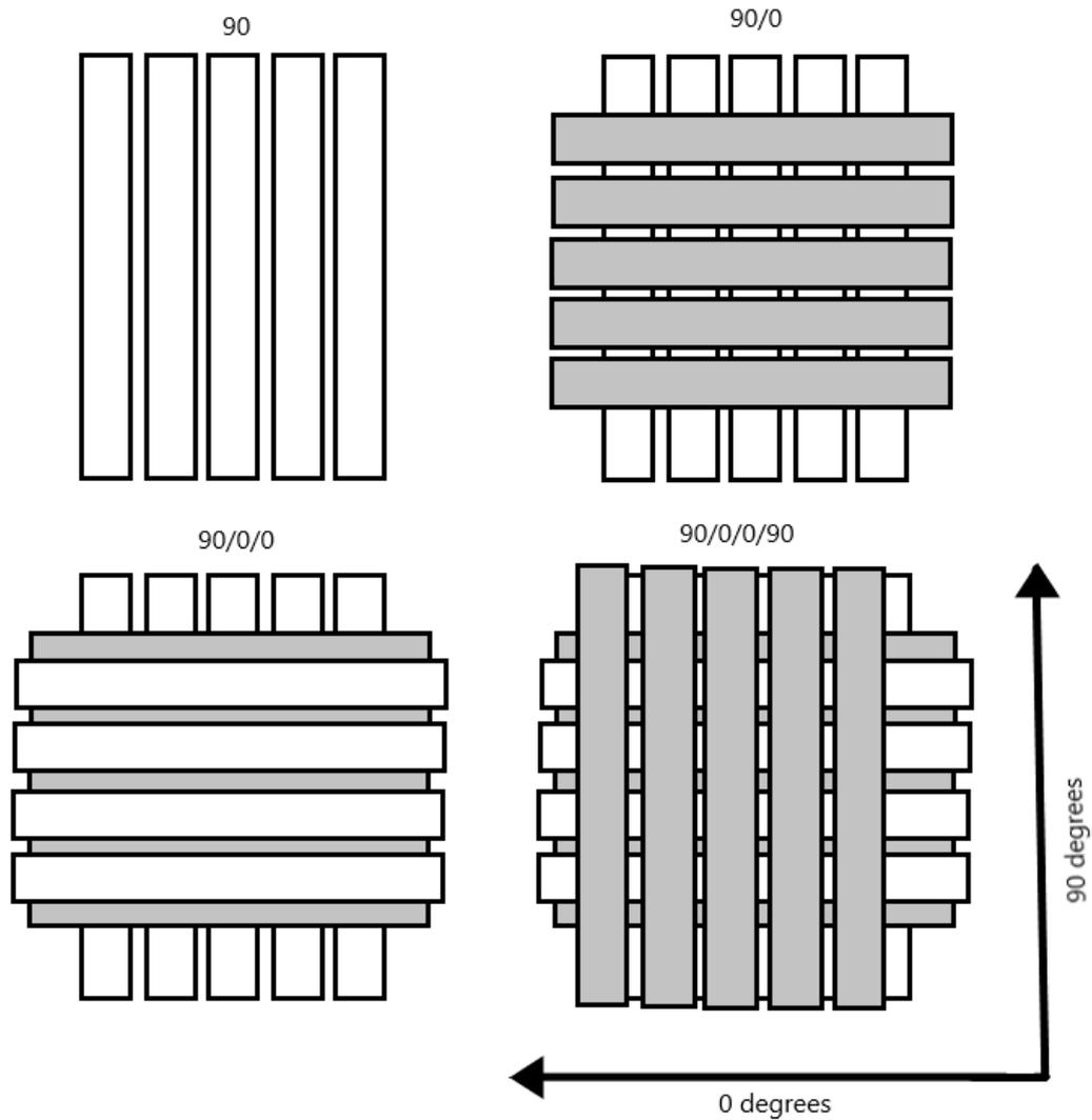
**Figure 6. Layer order and directions in the prototype panel of the thesis**
