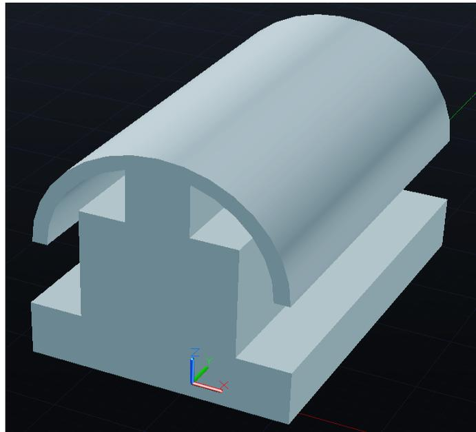
**Figure 4** The 3D model (AutoCAD) of the mould
