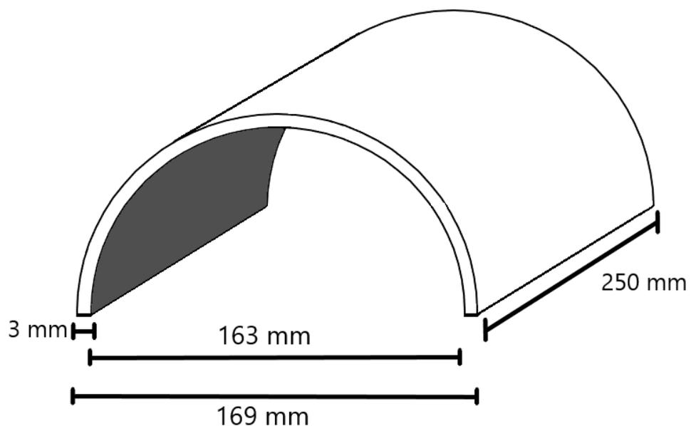
**Figure 2. Dimensions of the protective panel**
