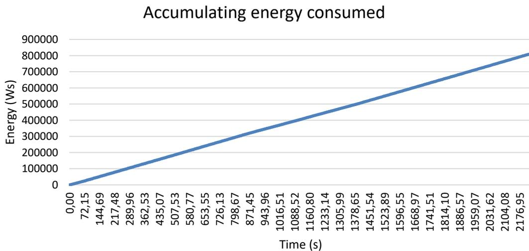
**Figure 8. The cumulative energy by integration of true power during the robot operation when laminating the prototype panel.**
