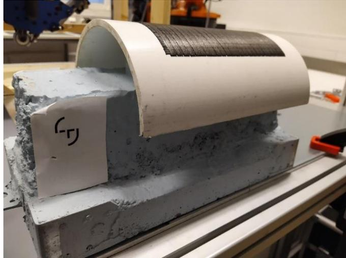
**Figure 3** The prototype mould and layers of pre-preg tape on it
