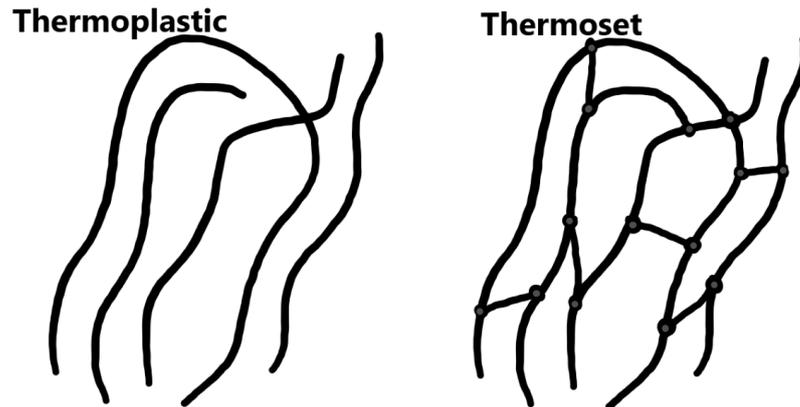
**Figure 1. The different structure of polymer chains in thermoplastics and thermoset polymers**
