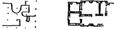
Fig. 11: After Le Corbusier; free plan vs. bearing wall, in Five Points of a New Architecture (1926).
