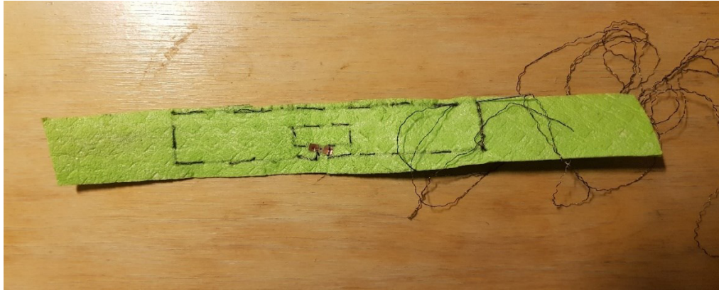
Figure 26. Construction of Passive UHF RFID moisture sensor tag by hand stitching in Material-3.
