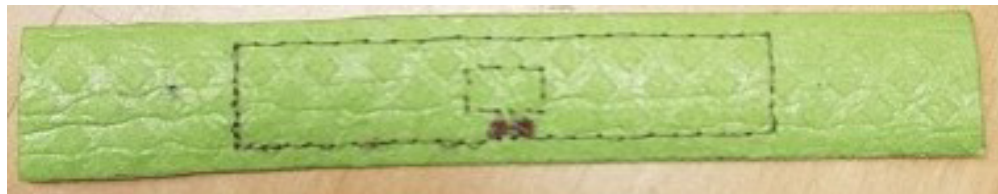
Figure 26. Construction of Passive UHF RFID moisture sensor tag by hand stitching in Material-3.
