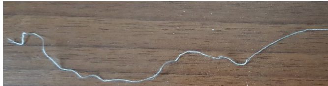
Figure 23. Soluble thread for evaluating the sensor in bending condition.
