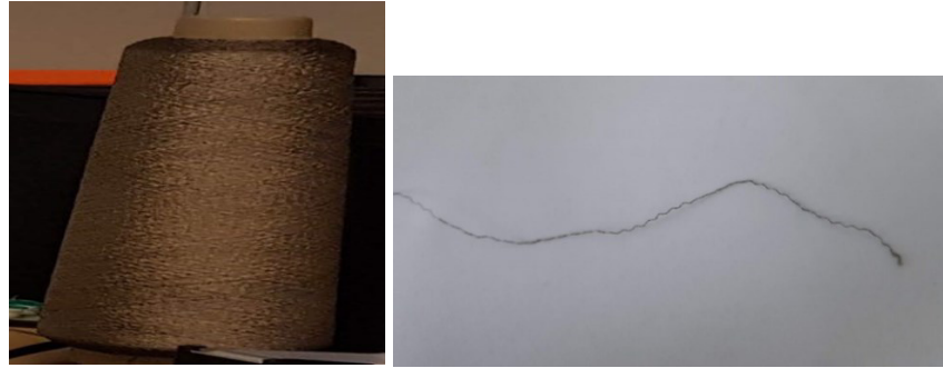
Figure 22. Conductive thread for construct the sensor.
