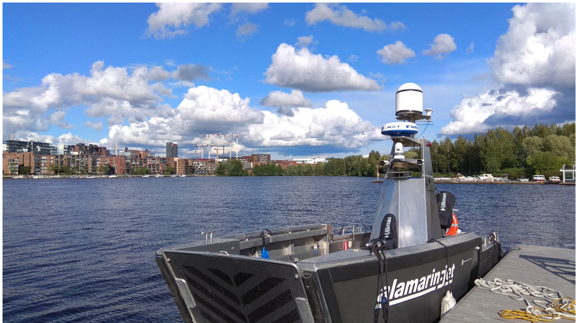
(b) Final implementation of the USV with the dome on directional antenna
