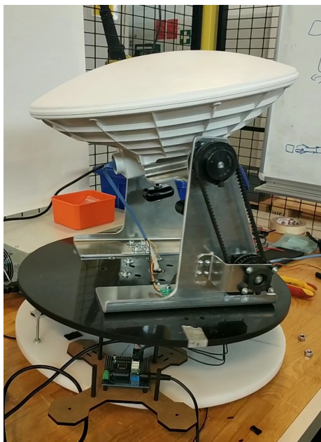
(a) Final mechanical structure for USV's directional antenna
