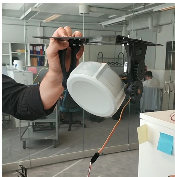
(b) Final mechanical design for mounting platform of UAV's directional antenna
