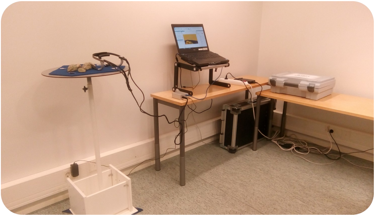
Figure 11. Stone Balancing Gaze Tracking Lab Setup: stones, standing table, Dikablis gaze tracker and Dell Precision 4800 (Windows OS) laptop.
