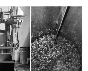
**Figure 1.** (a) Laboratory scale foam forming equipment; (b) nanocellulose-carbon nanotubes (NC-CNT) dispersion, pulp, and water mixture before foaming.
