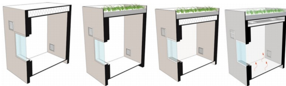
Fig. 4. Test cells with insulated traditional (cool) roof, non insulated green roof, insulated green roof and variable insulation green roof.
