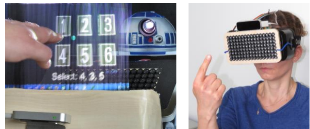
Fig. 5. Left: desktop-sized mid-air fogscreen with mid-air haptics [80] (©2015 IEEE). Right: mid-air ultrasound haptic feedback in front of a VR HMD [16].
