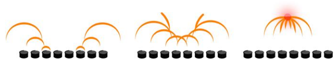
Fig. 1. This image sequence demonstrates the principle of focusing ultrasound from a phased array of eight transducers. The phase of each wave is offset such that they arrive at the desired point at the same time.
