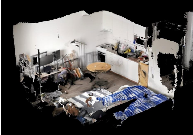
Figure 10. 3D model of a small apartment using Vonásek's 3D scanner using 2 cm resolution.
