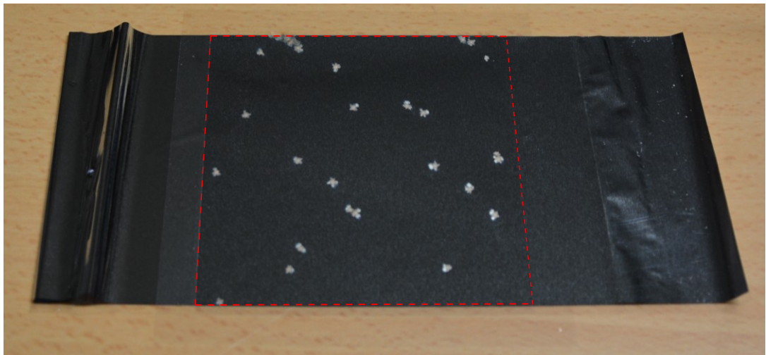
Figure 5.2.7. A photograph of a test capacitor after an endurance test demonstrating multiple self-healing breakdowns. The dashed red lines depict the active area.
