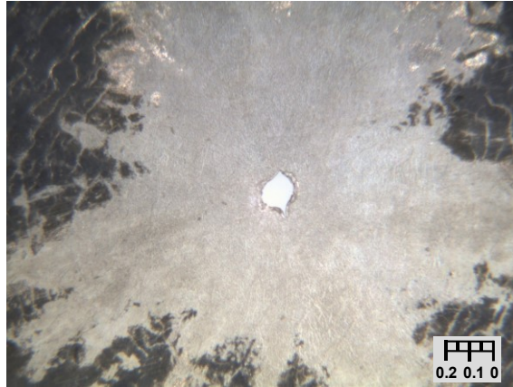
Figure 5.2.6. A microscope image of a self-healed breakdown. The scale bar is in millimeters [51].
