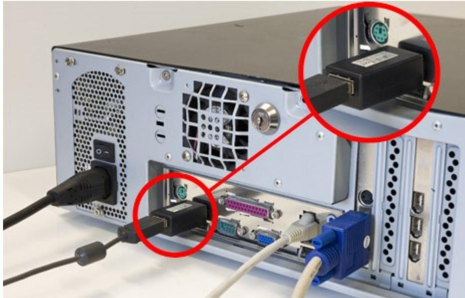
**Figure 1:** A typical example of a hardware keylogger is a USB hardware keylogger installed between the motherboard of the computer and the keyboard USB cable. For a regular computer user, it can be very hard to detect the keylogger just by a glance at the computer. Source: Wikimedia. [5]
