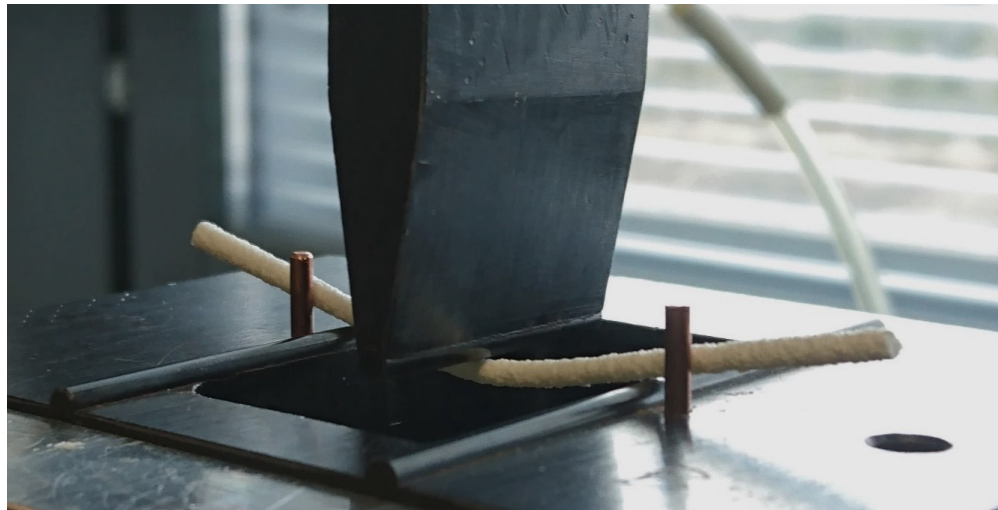
Figure 8. 3-point bending setup used in the study. Sample diameter ca. 2 mm, sample length 7 cm, loading radius 1.5 mm, bending span 32 mm, and cross head speed 5 mm min -1 .
