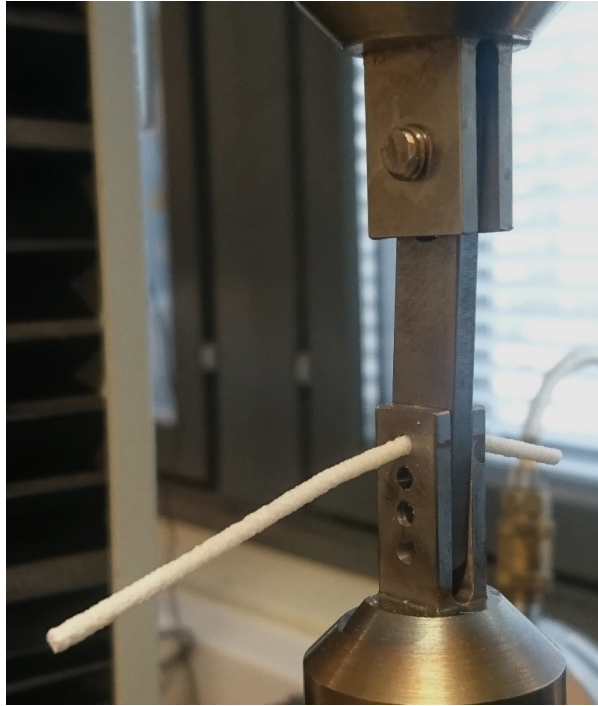
Figure 9. Shear setup used in the study. Sample diameter is ca. 2 mm and cross head speed 10 mm min -1 .
