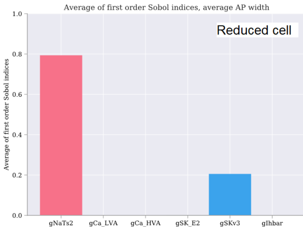
Figure 28: The average of the first order Sobol indices for average AP width in the reduced model. Here the uncertainty contributes mostly on the sodium conductance and less of potassium conductance.
