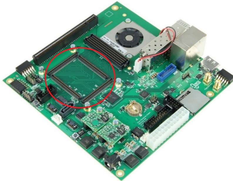
Figure 4. Overview of Trenz TEBF0808 carrier board with red circle encircling the connectors to which the MPSoC module should be placed (modified from source [14])
