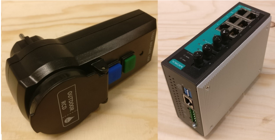
Figure 20: Test equipment: earth leakage circuit breaker and switch with a mirror port.
