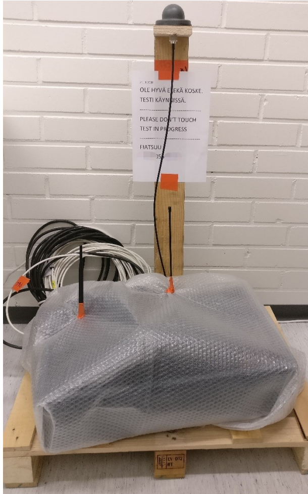
Figure 19: Master station on test bench wrapped to a homemade weather protection with long power cord and two Ethernet cables.
