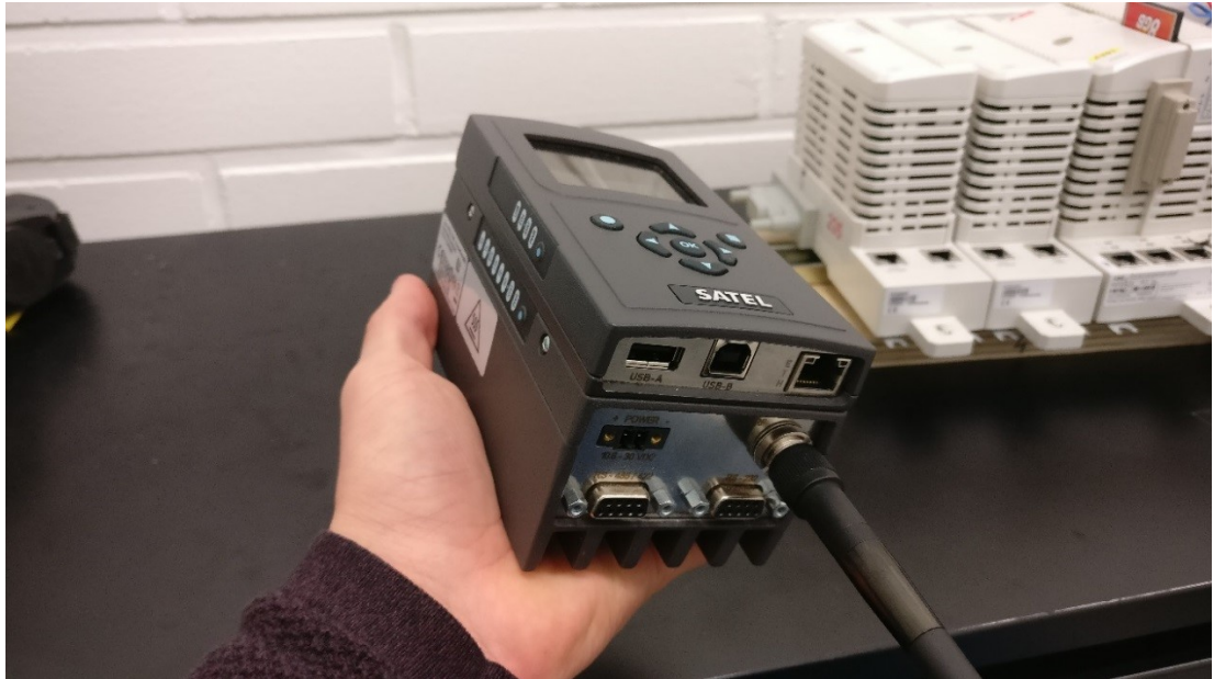
Figure 12: UHF IP Radio manufactured by Satel. The antenna showing is not the one used in tests.
