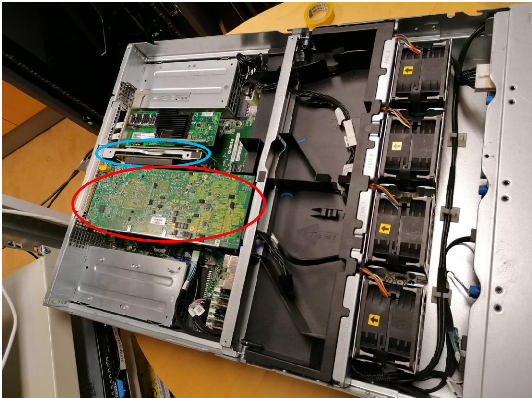
Figure 2.4 FPGA (red) connected to the CPU via PCIe (blue).
