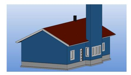
**Figure 11.** Screenshot from the Vertex BD program when the walls are stretched to the roof but there is no roof above some of the walls.
