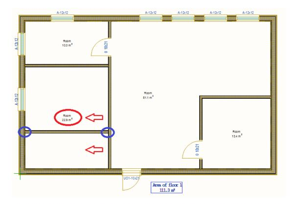
**Figure 13.** Example where there is no connection between the walls in either of the places in blue circles. This can be seen from room space. There should be room space note also in the lowest room.
