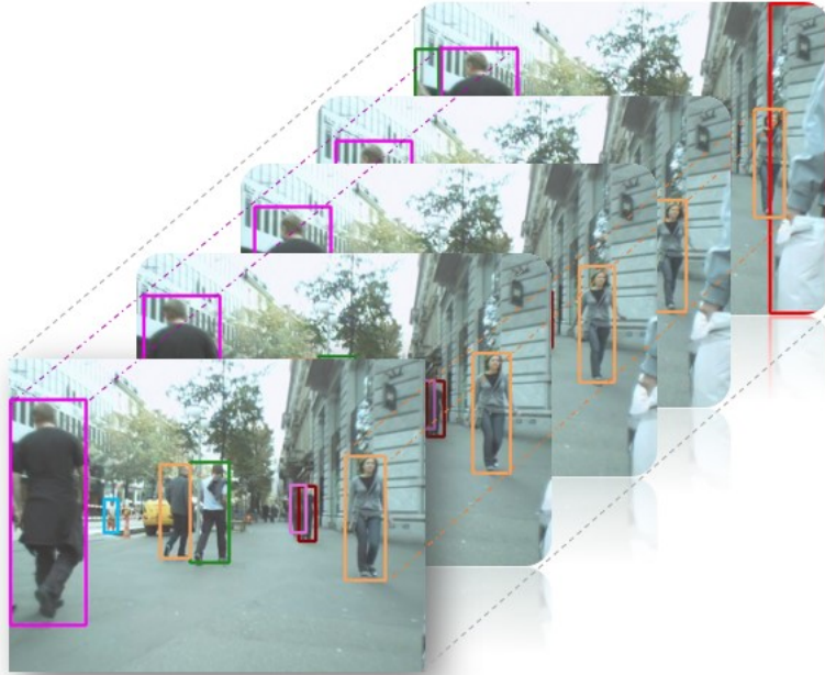
Figure 1. The ground-truth MOT result from MOT17DET [21]. They are selected as the five subsequent frames and organized following the time stamp.
