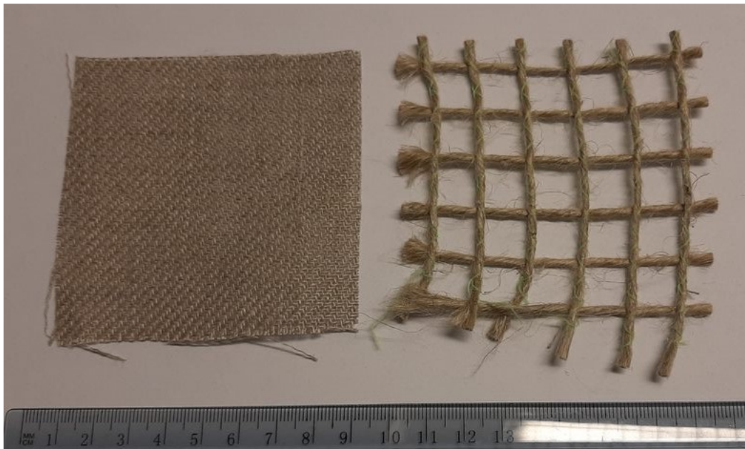
Figure 3.2: Woven flax fibre fabric and a piece of Power Ribs ® -fabric used in the thesis
