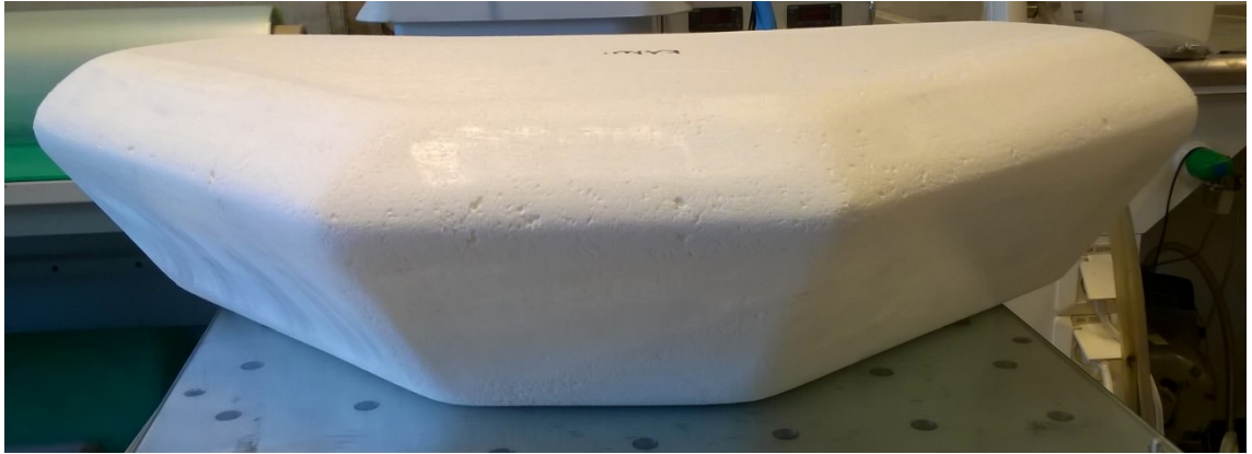
Figure 3.28: Fabricated EPS mould for the hull in this thesis for a CRU prototype.
