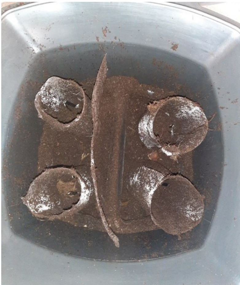
Figure 3.16: Compost bin being almost full during the loading process of medium and specimens.
