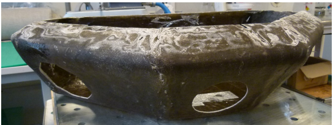
Figure 3.33: The CRU hull after finishing treatments to smooth outer surfaces.
