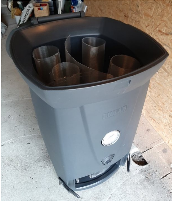
Figure 3.10: The compost bin used for the soil burial testing of polymer and composite specimens
