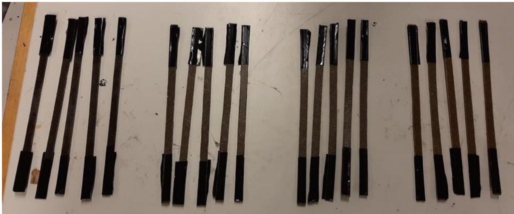
Figure 3.19: The composite tensile specimens after the composting. From left to right: flax epoxy, flax PLA, flax PLA+rosin, and rosin treated flax PLA+rosin.
