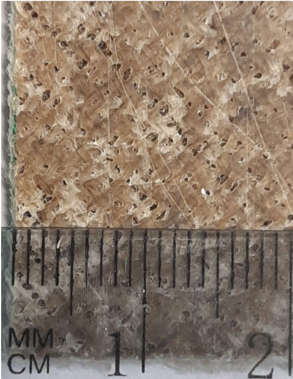
Figure 4.2: A close-up image from the surface of a RtFPR laminate.
