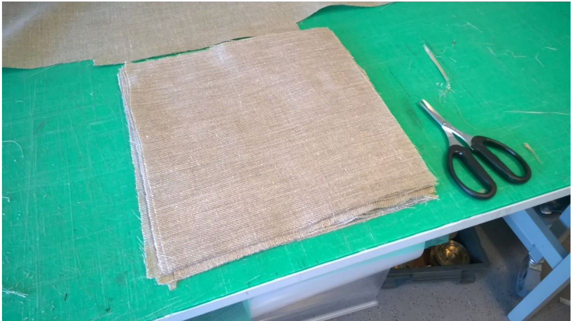
Figure 3.5: A stack of 30x30cm plies of the flax fibre fabric.
