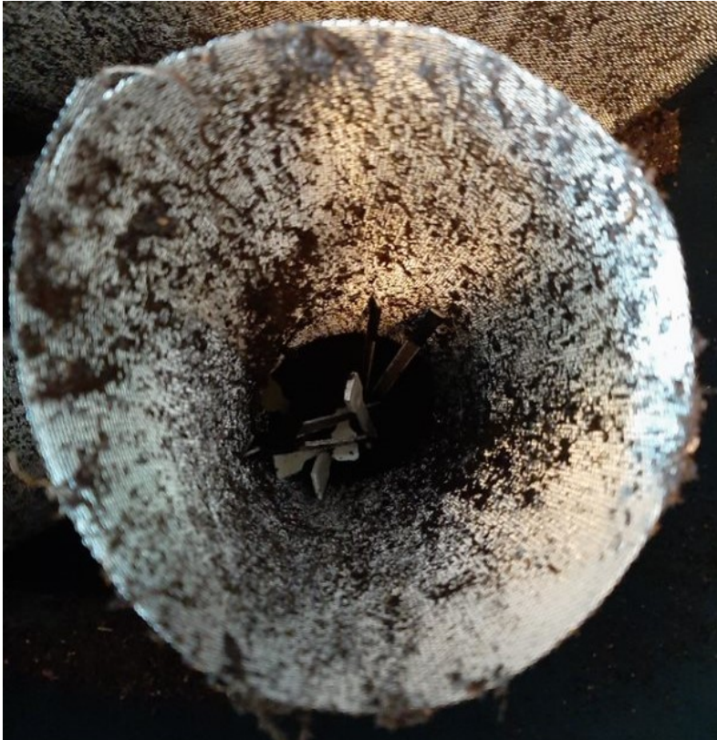
Figure 3.17: One of the stainless steel mesh tubes after placing in a set of specimens.
