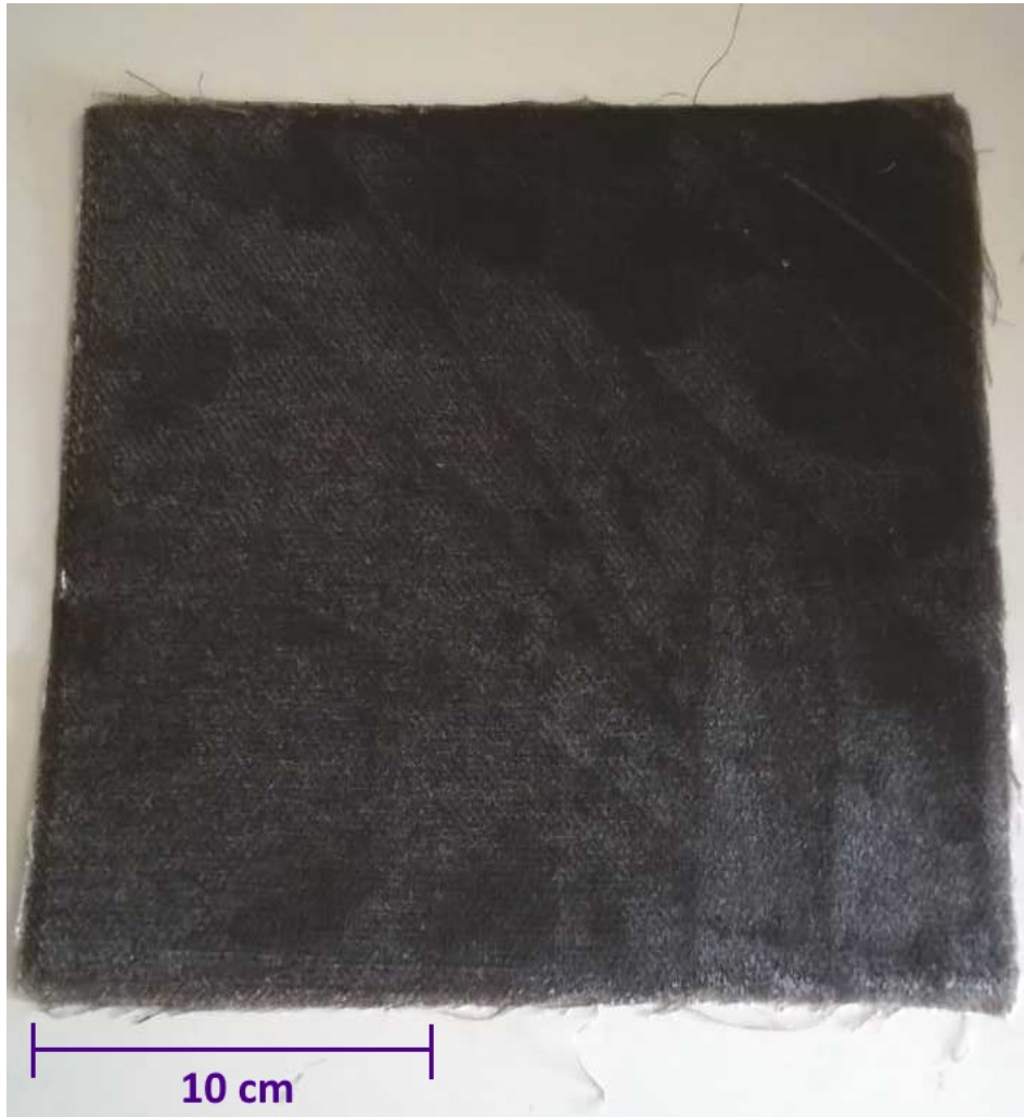
Figure 3.9: The trial laminate number 2 with fully impregnated layers of flax and close to optimum thickness for testing purposes.
