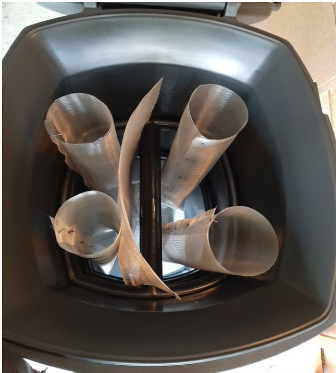
Figure 3.11: The compost bin from the inside showing the stainless steel wire mesh separator tubes and the wall
