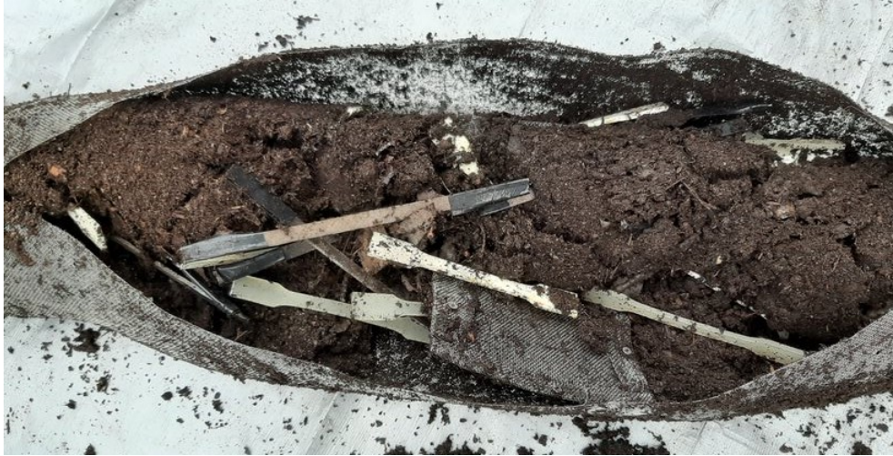
Figure 3.18: One of the steel tubes, containing the compost medium and specimens at the time of extraction from compost.
