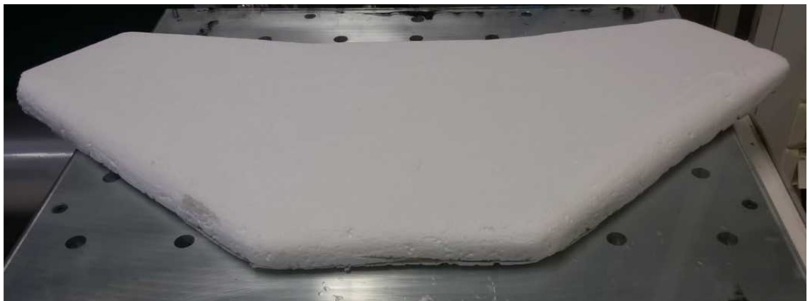
Figure 3.29: Fabricated EPS mould for the top cover in this thesis for a CRU prototype.
