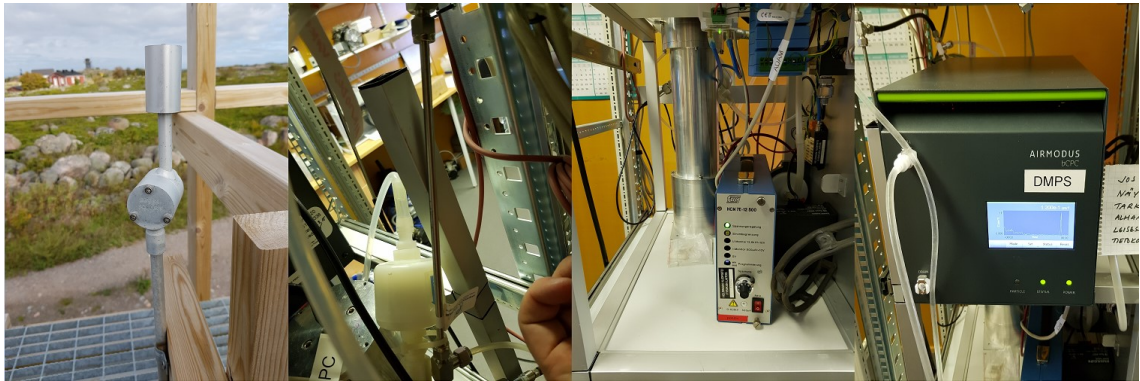
Figure 3 The pictures of the measurement setup at the atmospheric measurement station of Utö in September 2019. The instruments from left to right are: The PM_{2.5} inlet, the nafion dryer, the DMA of the DMPS, and the CPC of the DMPS.
