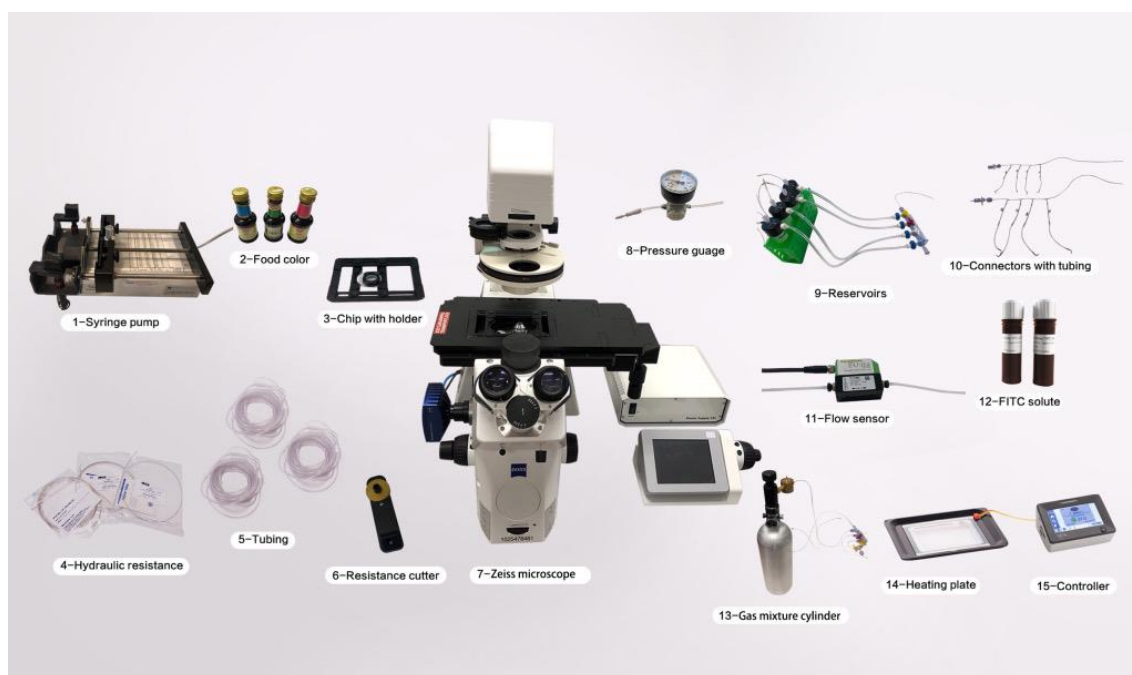
Figure 23. Critical components of two microfluidic platforms
