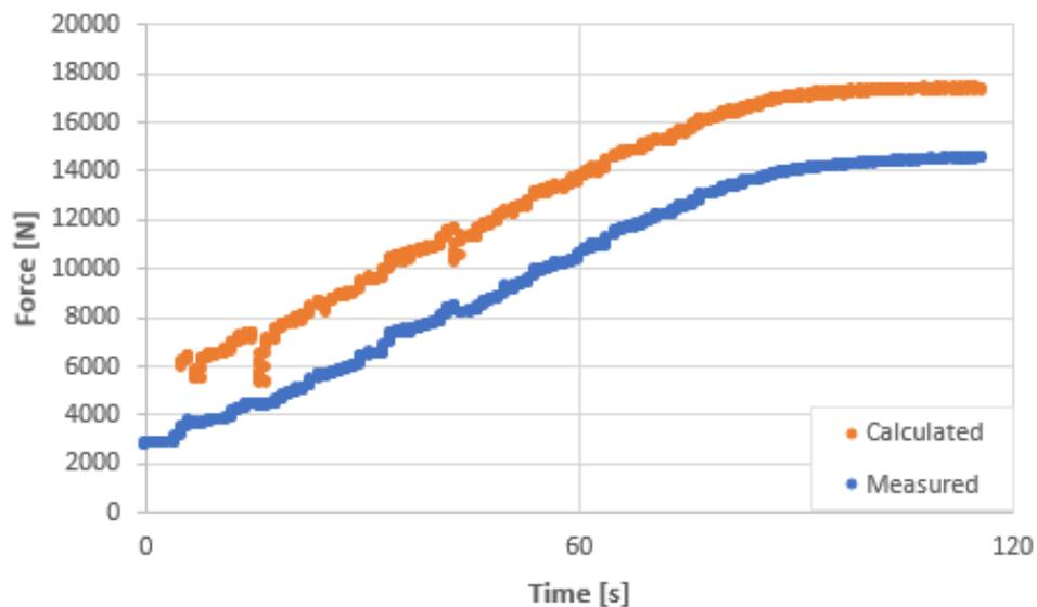
**Figure 27.** Measured and calculated force of the 20-bar performance test.
