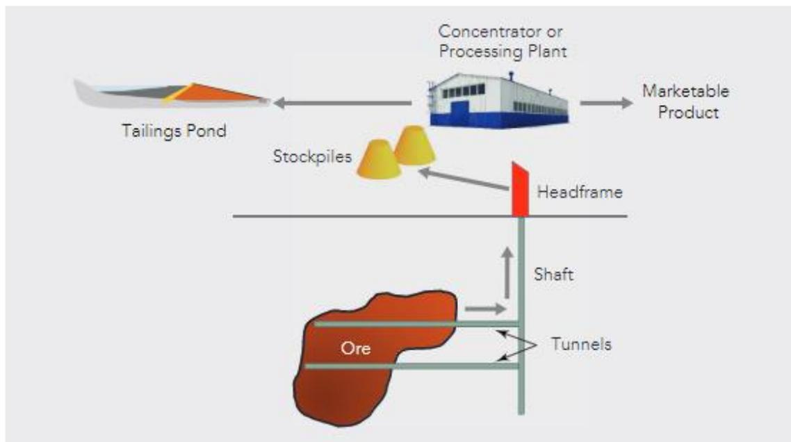
**Figure 1.** Typical configuration of an underground mine [10].
