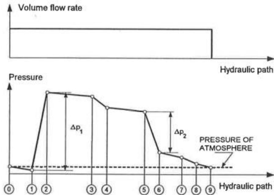
**Figure 8.** Volume flow rate and pressure of the hydraulic system [23].
