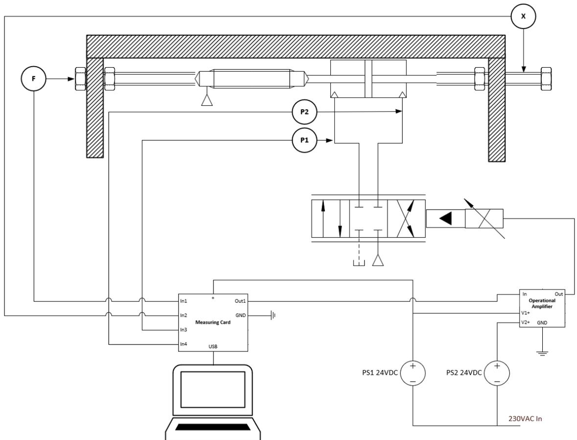
**Figure 22.** *Measuring setup and servo valve control.*
