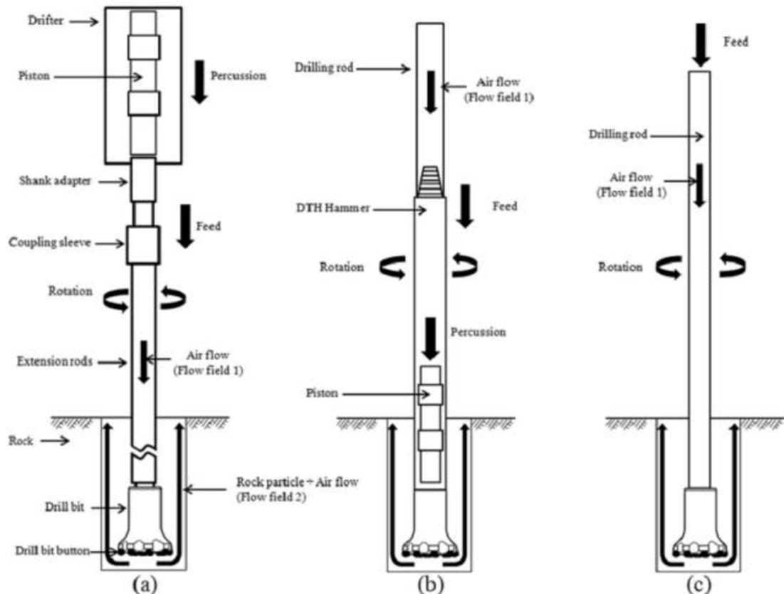
**Figure 18.** Three methods of rock drilling. (a) Top hammer drilling. (b) Down-the-hole drilling. (c) Rotary drilling. [64]
