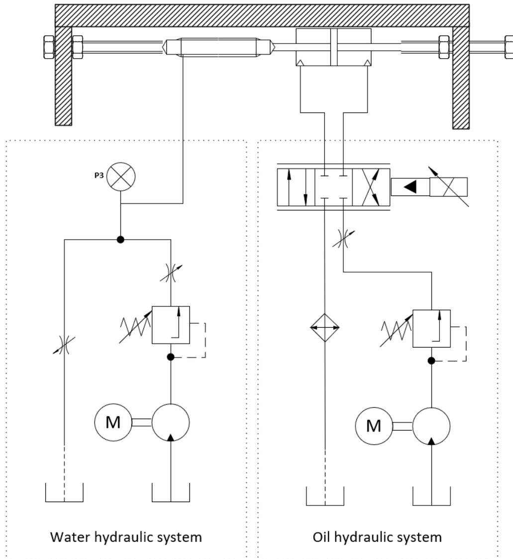
**Figure 21.** Test bench and its hydraulic system.
