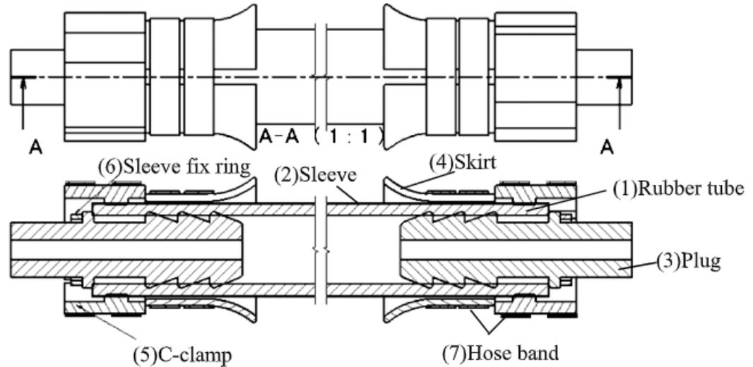
**Figure 12.** A typical structure of a HAM [39].
