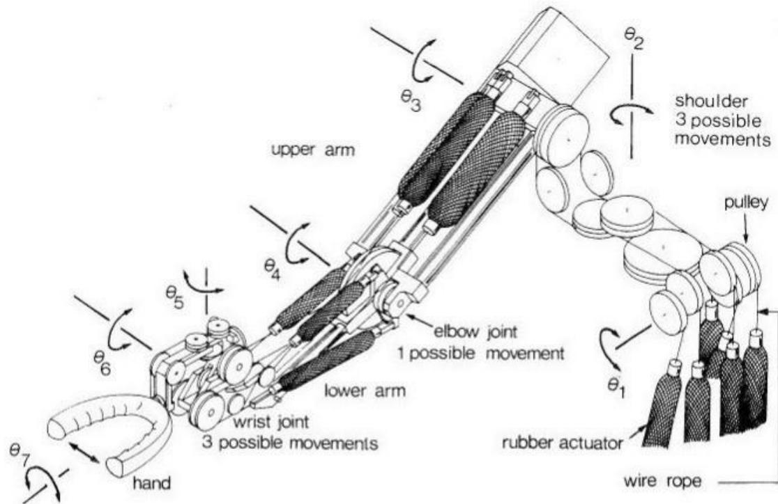
**Figure 11.** Bridgestone's and Hitachi's robot arm [31].
