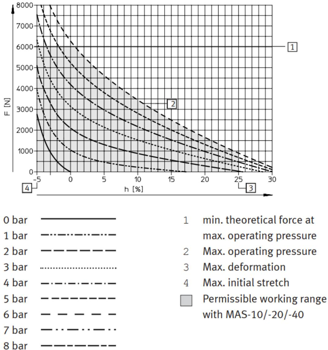
**Figure 20.** Force and displacement graph of the Fluidic Muscle [45].
