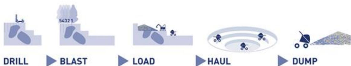
*Figure 3. Open-pit mining cycle [8].*
