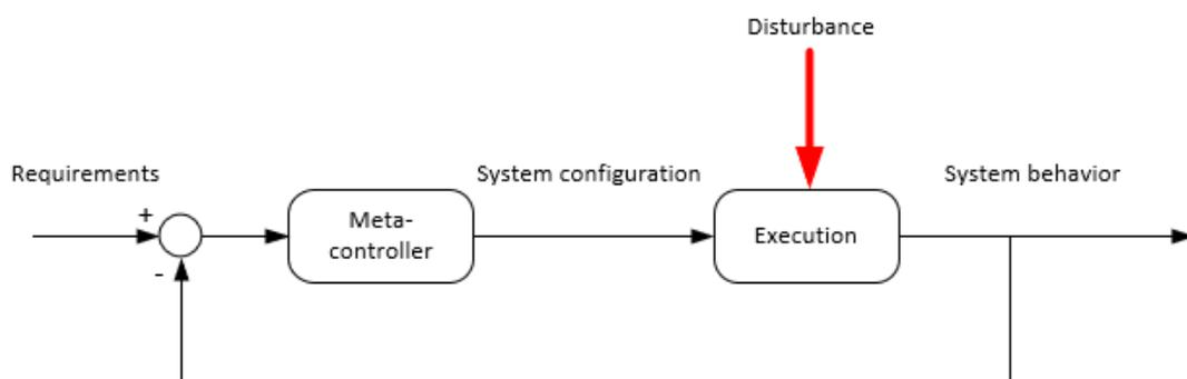
**Figure 17.** Resilient control architecture.
