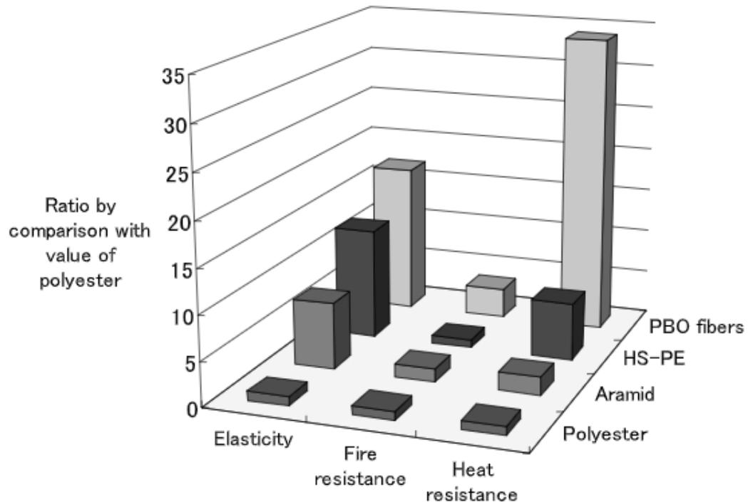
**Figure 14.** Elasticity, fire resistance and heat resistance compared to polyester [39].
