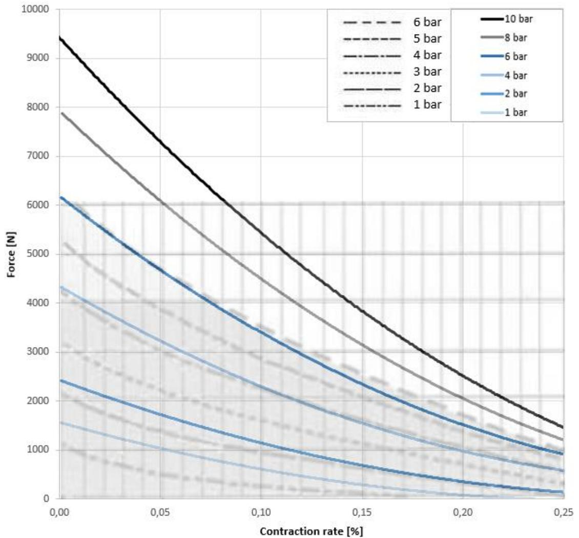
**Figure 26.** Comparison of FMB's test results and given graph.
