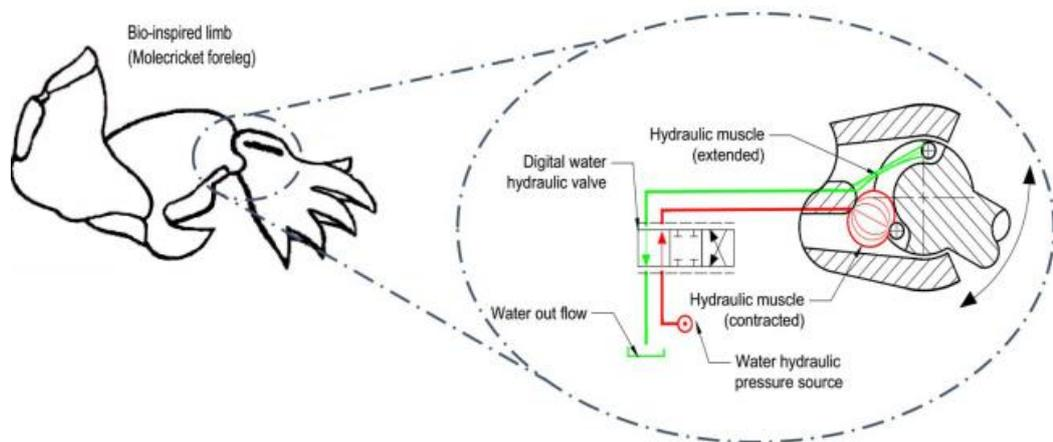
**Figure 5.** Example of water hydraulic actuator-based limb and its system [1].
