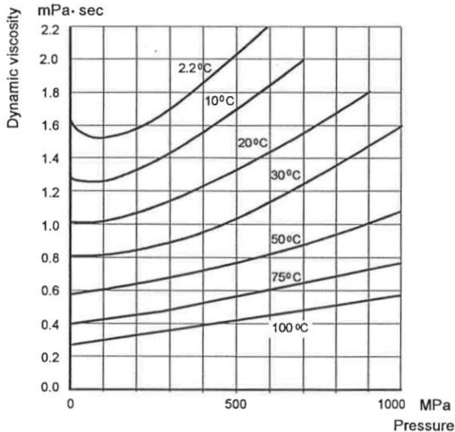
**Figure 6.** Viscosity's dependency to temperature and pressure of the water [23].
