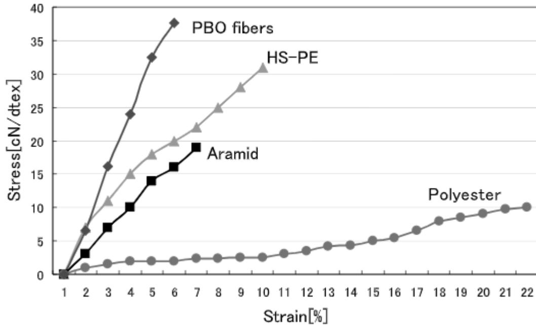
**Figure 13.** Stress-strain plot of different sleeve materials [39].
