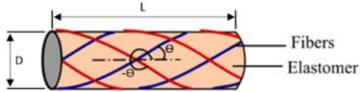
**Figure 15.** The fibres and elastomer of a FREE actuator [40].
