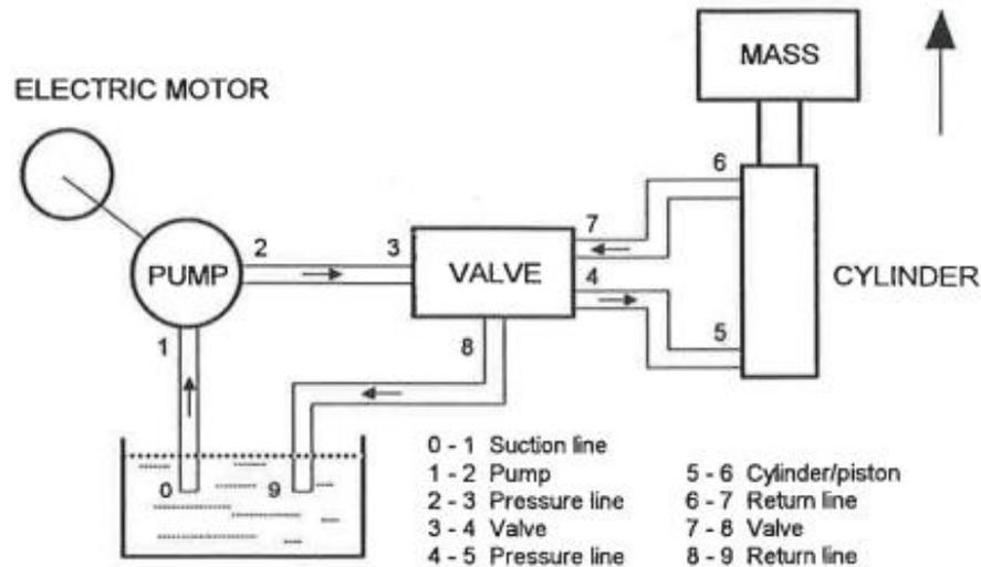
**Figure 7.** A simple hydraulic system and its components [23].
