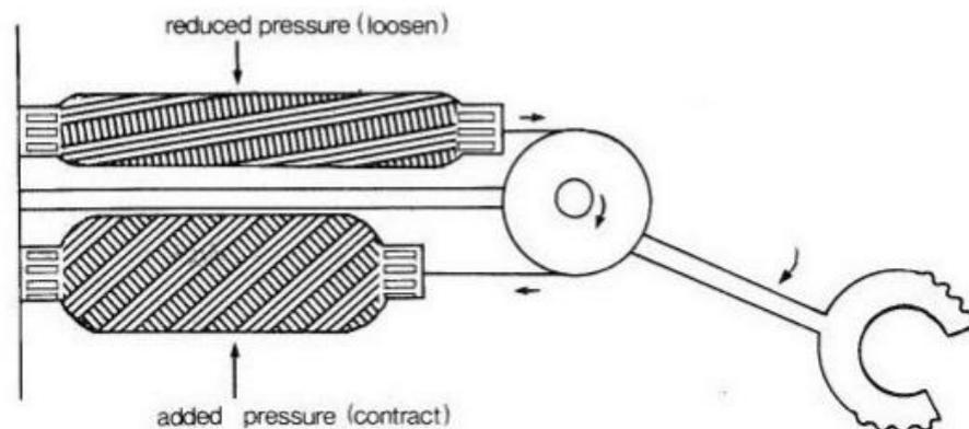
**Figure 10.** Bridgestone's artificial muscles and their operation principle [31].
