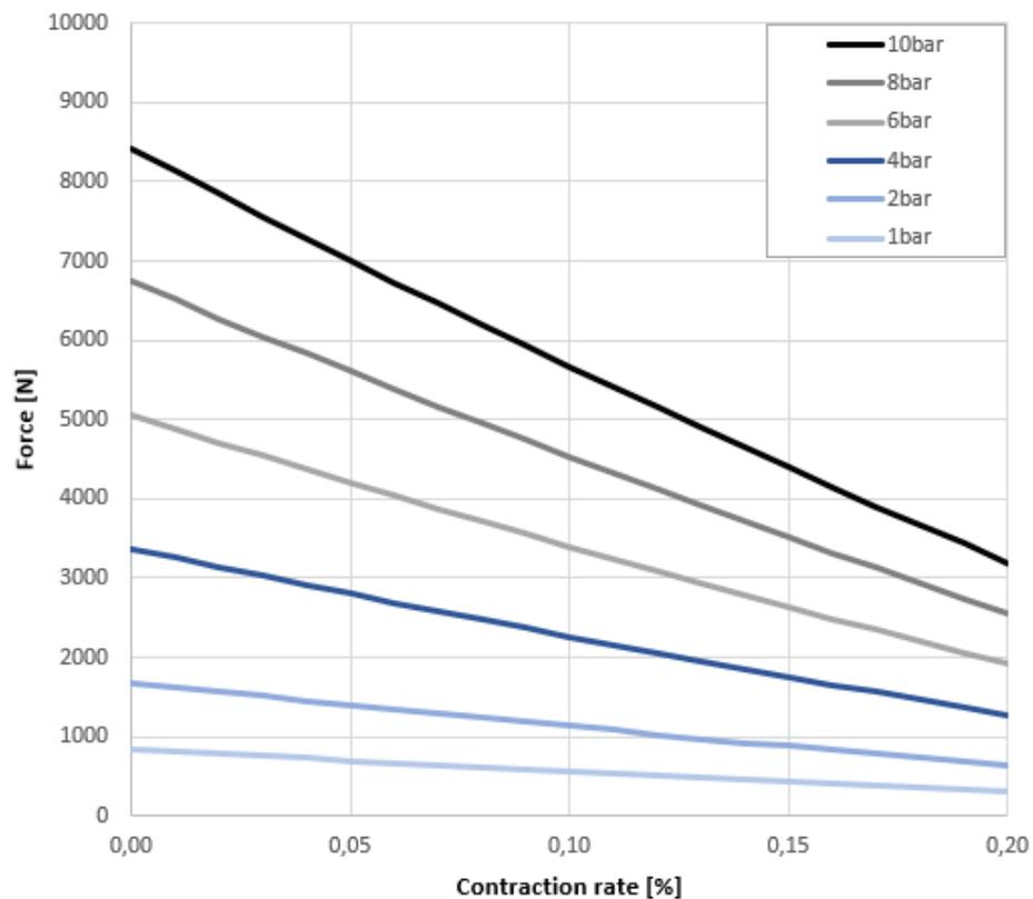
**Figure 28.** HAM's predicted output force as a function of contraction rate.
