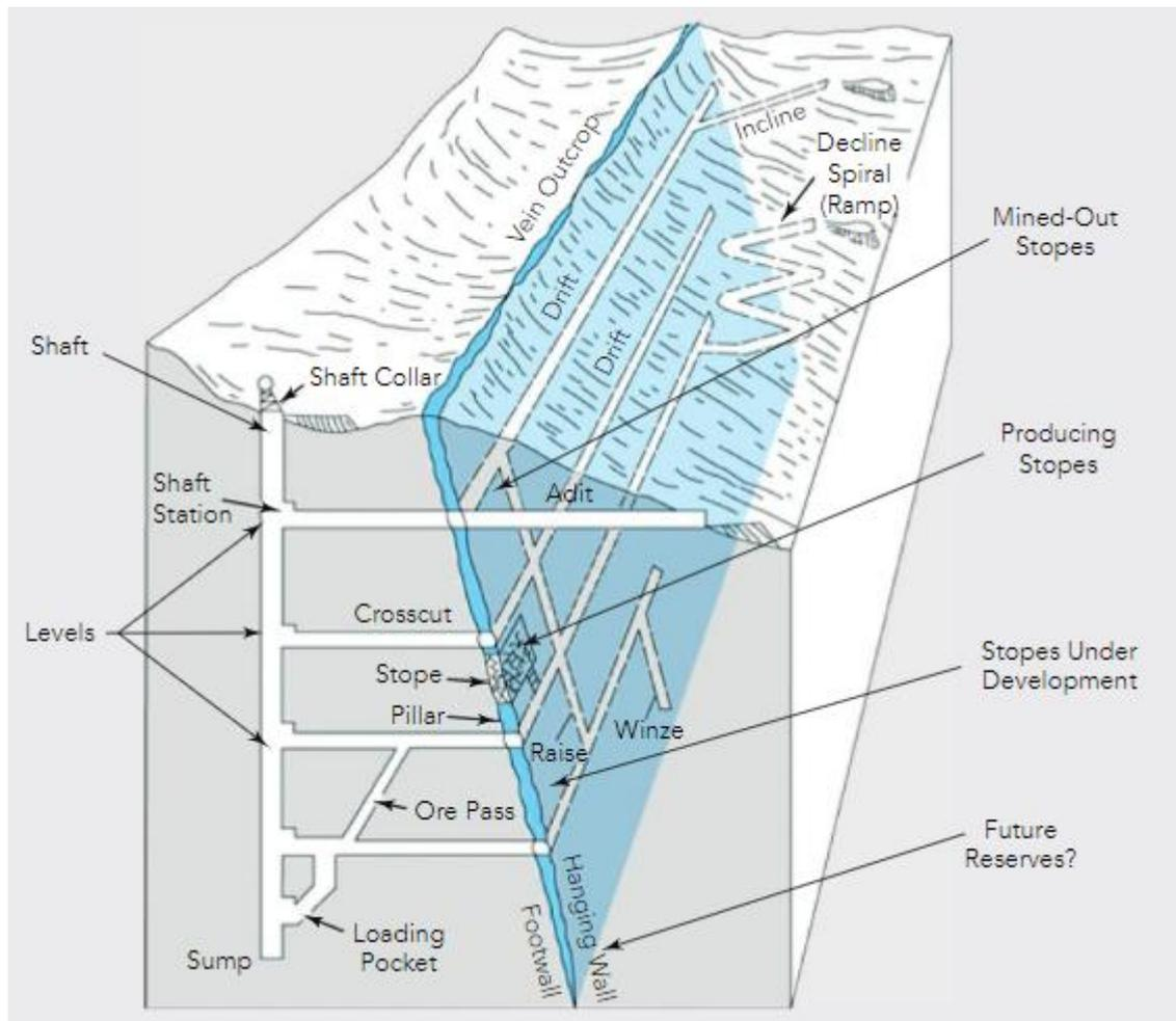
**Figure 2.** *Underground mine demonstration and vocabulary [10].*
