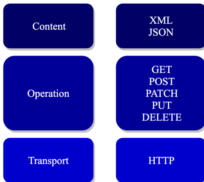
Figure 9. RESTCONF protocol stack
