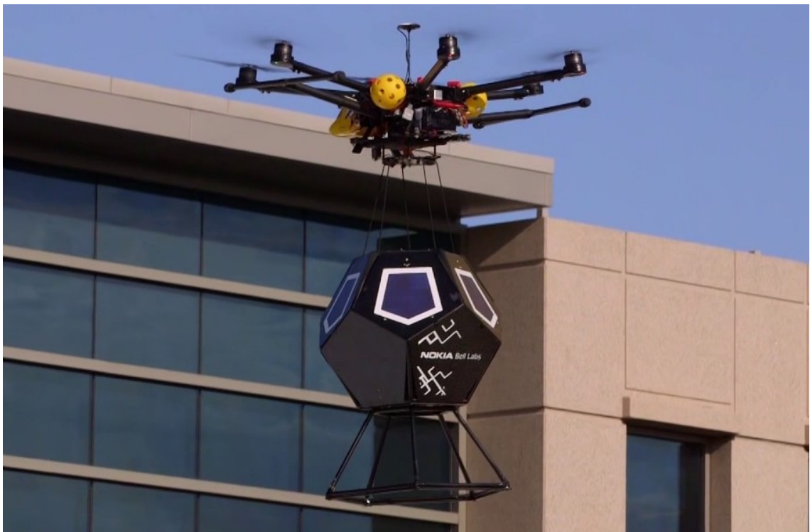
Figure 1.2. UAV acting as BS carrier (borrowed from [15]).
