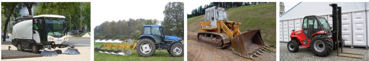
Figure 2. Off-Road Machines with Tools offside of the Vehicle's Pivot Point without an Additional Hinge
