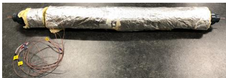
Photo 1. The heat-resistant vinyl chloride pipe covered with thermal insulation material
