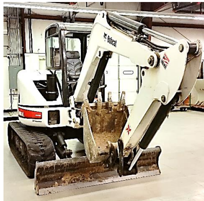
Figure 4. DC prototype Bobcat 435 mini excavator at Maha Fluid Power.
