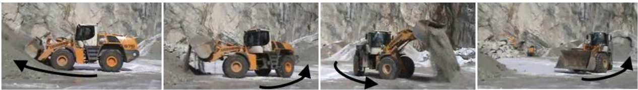
Figure 2. Wheel loader's y-cycle
