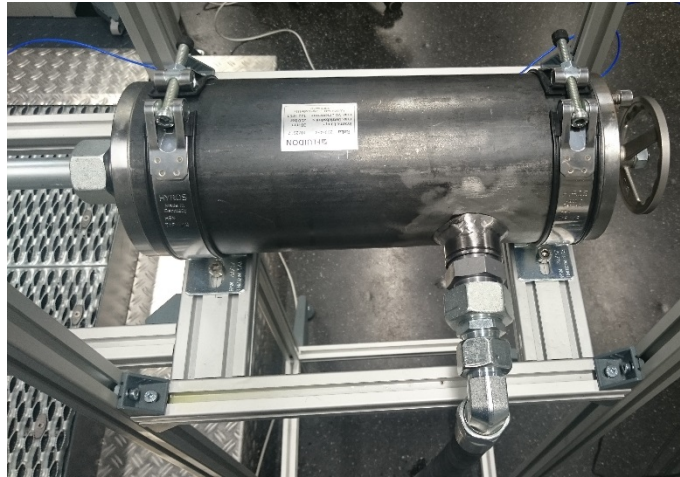
Figure 17. Low-reflection line terminator (RaLa)
