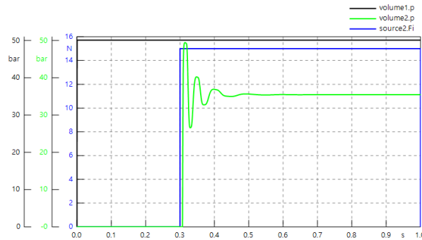
Figure 9. Step response result(supply pressure: 50[bar], Input attraction force: 15[N])
