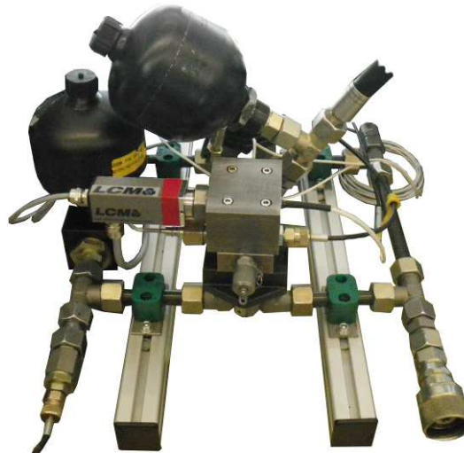
Figure 2 Test rig with valve, power electronics, valve block and accumulators
