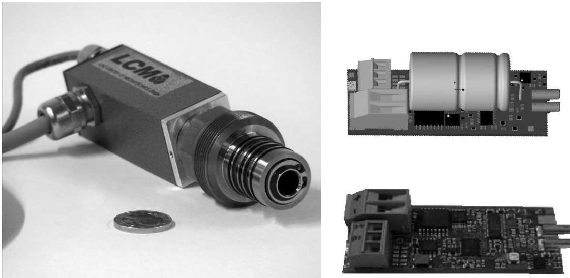
Figure 1. Complete prototype valve (including the integrated electronics in the (left) and 3D model and the electronic board (right)
